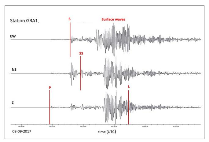
**Figure 5.7:** Three component seismogram of the magnitude 8 event offshore Mexico (08.09.2017, 04:49:21 UTC, Ms 8.3) recorded at station GRA1 of the Gräfenberg array. The SRO-LP filtered seismograms show the body and surface waves as well as identified and picked phases.
