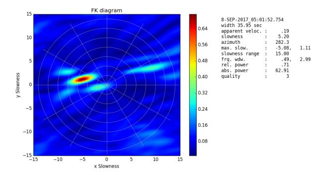
Figure 5.4: Result of the f-k analysis for the P wavetrain of an event offshore Mexico (08.09.2017, 04:49:21 UTC, Ms 8.3) recorded at the Gräfenberg array. The inferred slowness and azimuth can be used to backtrack the ray and determine the epicenter.
