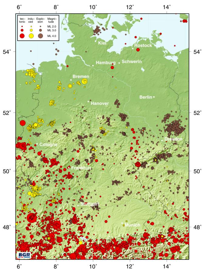
**Figure 5.3:** Seismic events with magnitude 2.0 and above in Germany and adjacent regions in the recent 20 years (1998-2017). The tectonic events, induced events, and explosions are colour coded. The different magnitudes of the events correspond to the size of the circles.
